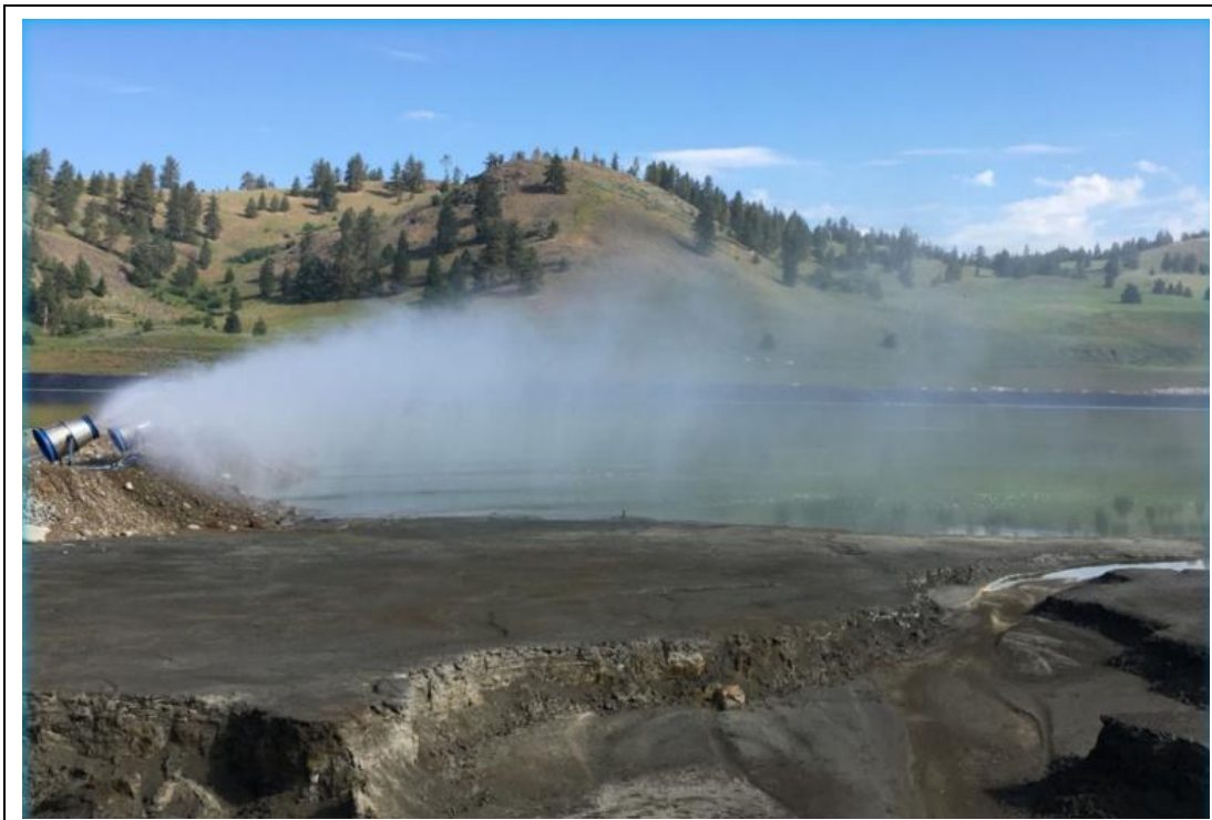
Figure 5-7 Landshark 2.0 Evaporator from Resource West Inc.
